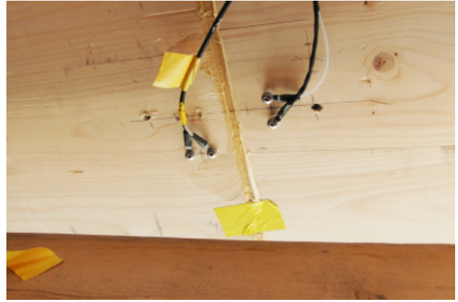
Measuring tool for checking the deformation behavior under changing wood moisture
